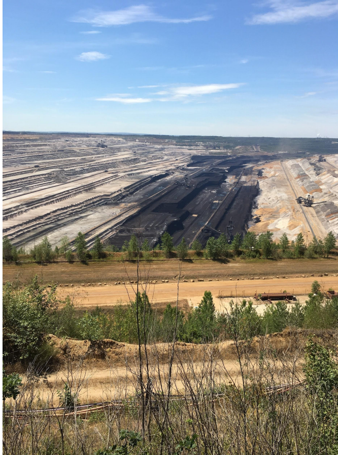
Figure 2. View of Hambach Mine from a lookout point. The sought-after lignite is visible as a black-colored substance at the bottom of the mine.
